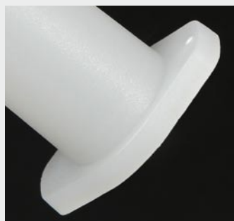
Part with 0° gating point on flange produced in an 8-drop test mould
