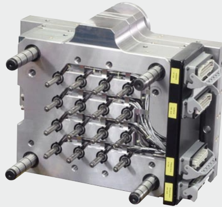
Compact hot half with valve gate system. Joint drive with all valve pins fixed in actuator plate
